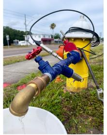
The new p-CAT<sup>™</sup> Infinity methodology is specifically designed for inspections of 6-inch to 16-inch mains where the main doesn't need to be isolated and equipment can be deployed via fire hydrants and 1-inch taps.
