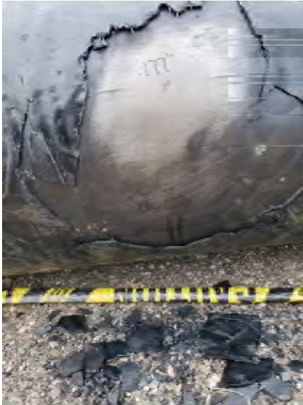
Figure 5 & 6 – Outer Coating Removal to Check Bonding (orange color is from paint)
