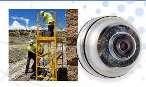
Hydromax USA team launches Nautilus, typically via insertion at a vertical valve, and the sphere is released into the flow of the water. Nautilus creates an audio recording as it moves with the flow of water.
